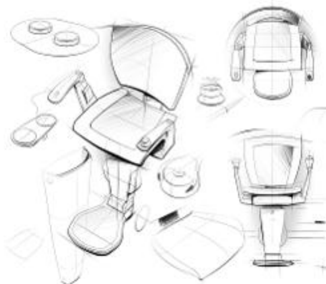
[5.35] Rendering of monorail with old armrest principle and sketch of altered design
