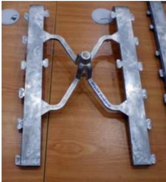
[4.17] First out of tool of magnesium front legs and [5.18] tool of the PP-seat
