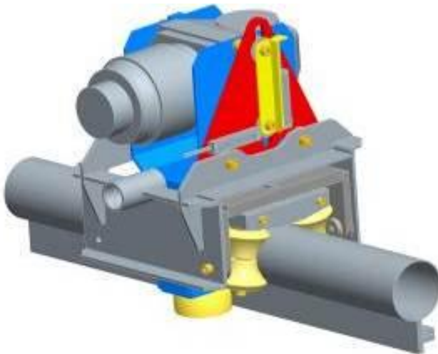
[5.19] Motor section slides in between the two wheel sections
